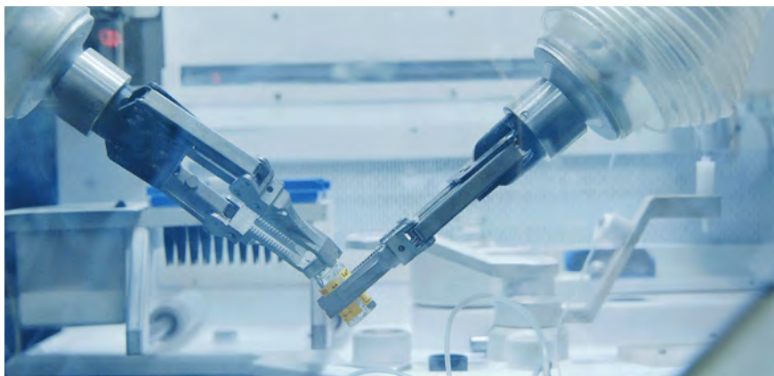
Radiolabeling (II): a manipulator in the process cell
